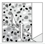
Positioning concrete forms on concrete surfaces. Leave in place, grey polyethylene is non rusting, nearly invisible and non-conductive.
